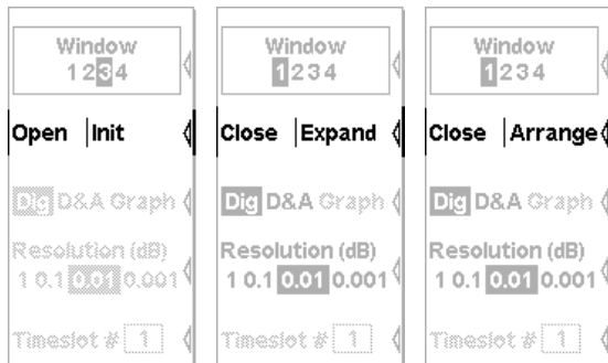
Fig. 4-24 Windows menu, softkeys for controlling the windows
