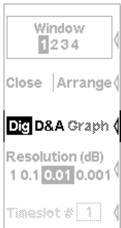
Fig. 4-25 Window menu, softkeys for controlling the display mode
